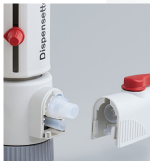
Valve system designed without seals
