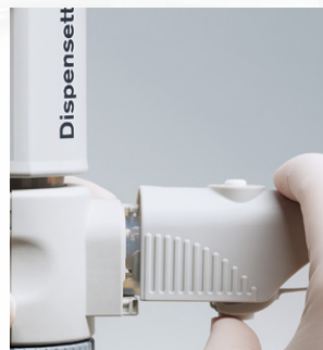
Simple-to-mount discharge tube
