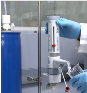
Remote Dispensing System for Drum Dispensing
