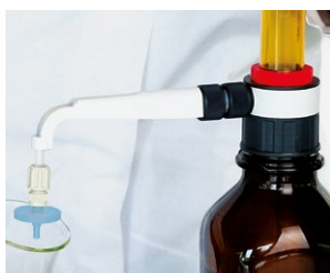
Sterile filtration of media directly from the bottle using the discharge tube with Luer-Lock connection
