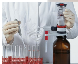
Serial dispensing with flexible dispensing tube
