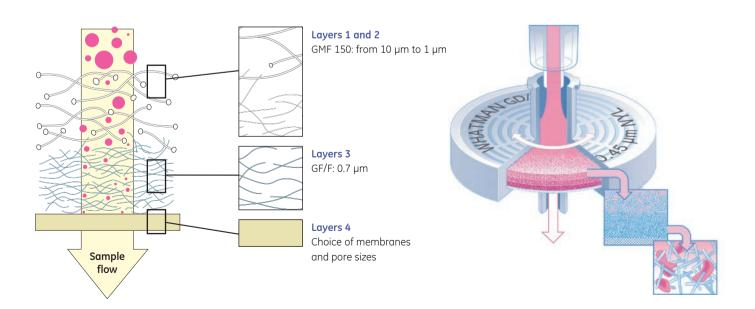
Whatman GD/X Syringe filters contain several filtration layers that substantially reduce blockage and increase volume throughput.
