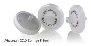
GMF 150 and GF/F are produced from 100% borosilicate glass microfiber. The graded density GMF 150 filtration medium has a coarse top layer meshed with a fine bottom layer that retains particles to 1.0  $\mu$ m. A GF/F filter then retains particles down to 0.7  $\mu$ m. The prefilter stack ends with a final membrane filter.
